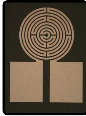
A diamond RTD temperature sensor with patterned metallization for a rapid response time
